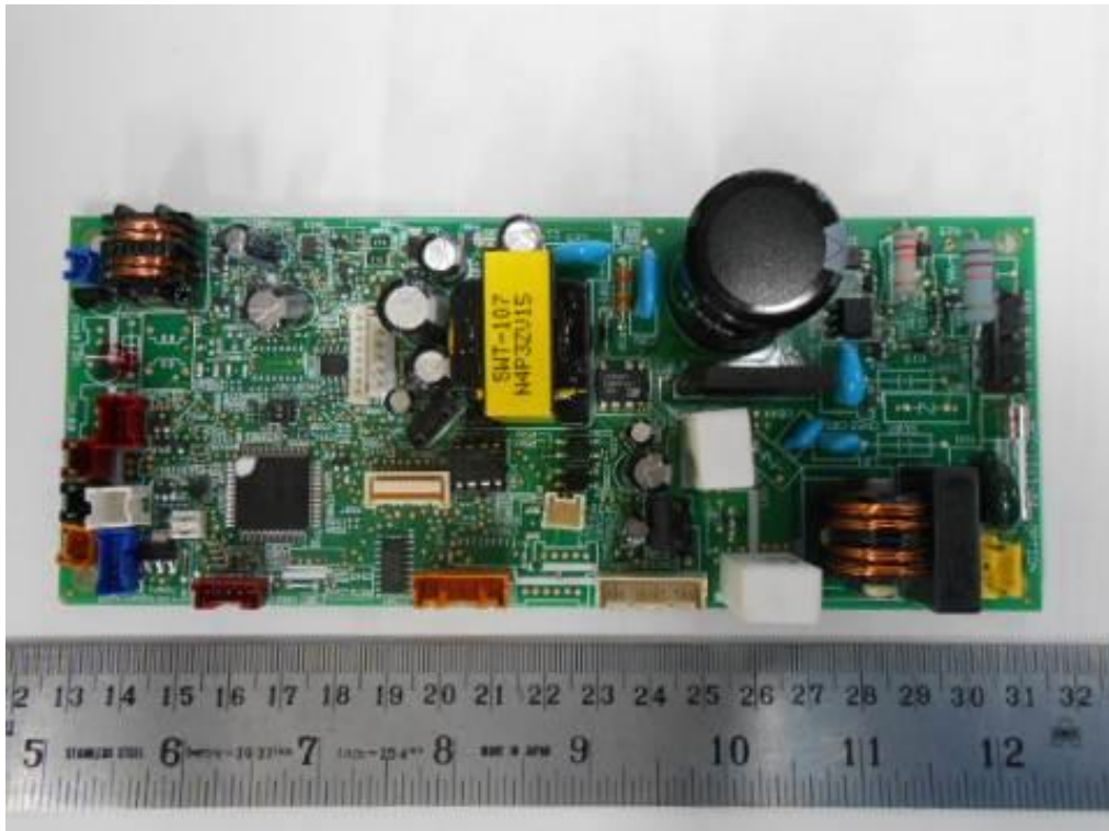
33. RAV-HM1601CTP-E, Control PCB components side. (Representative)
