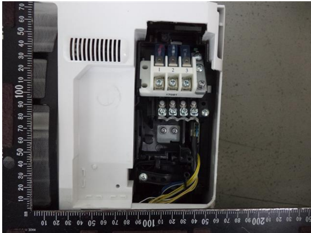
13. Terminal block, High wall RAV-HM801KRTP-E (Representative).
