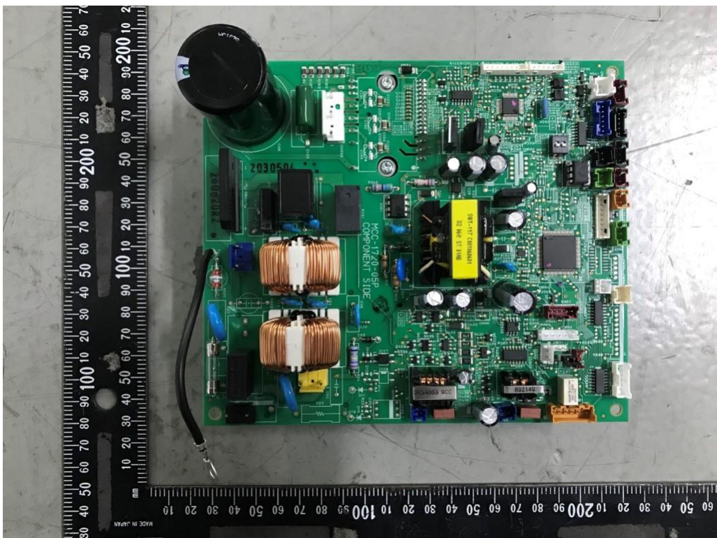
8. PCB, Duct type RAV-HM1601BTP-E (Representative).
