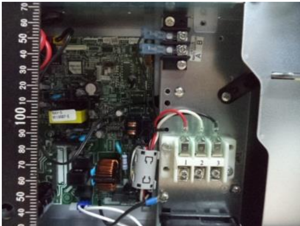
6. Terminal block, Duct type RAV-HM1601BTP-E (Representative).
